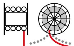
**Cylindric drum (multi spires multi layers random wound)** it is the cheaper reel but it doesn't guarantee the control over the layers of cable: the cable could be stacked, for example, on one side of the drum.
