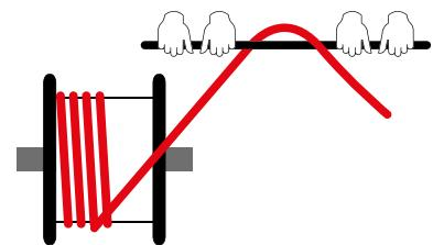
Aristoncavi's cables are produced with S stranding direction. In this case we recommend to start winding the cables, on the reeling drum, from the left side of reel as shown in the pictures:
