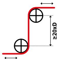
For a large diameter cable it would be better to use rollers to reduce the friction with the sheath during the change of direction.
