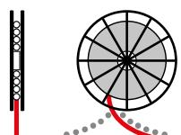
**Multispiral drum (multi spires single layer)** used in case of long cable lengths. It is important to ensure that the guide mechanism doesn't damage the cable during unwinding, for example: avoiding anomalous rub against the surface of the previous spire or irregular twisting. It is advisable to use maximum two layers to allow the thermal balance.
