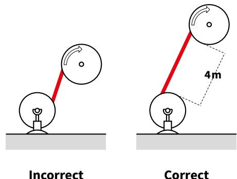
It's necessary to be careful during the transfer of the cable because it could have a residual torsion from the beginning, before to start its real application.
