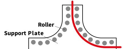
If sheaves are used, it is important to have a flat surface profile, to avoid unwanted rotations or twisting caused by the continuous clash with the sides of the sheave. In any case, the width of a cradle or that of a roller, should be 10-15% larger than the outer cable diameter to allow a correct running.
